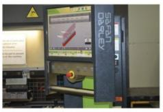
≫ The graphic interface on the touchscreen control provides the operator a visual representation of what is happening during the job, even the location of the backgauge.
