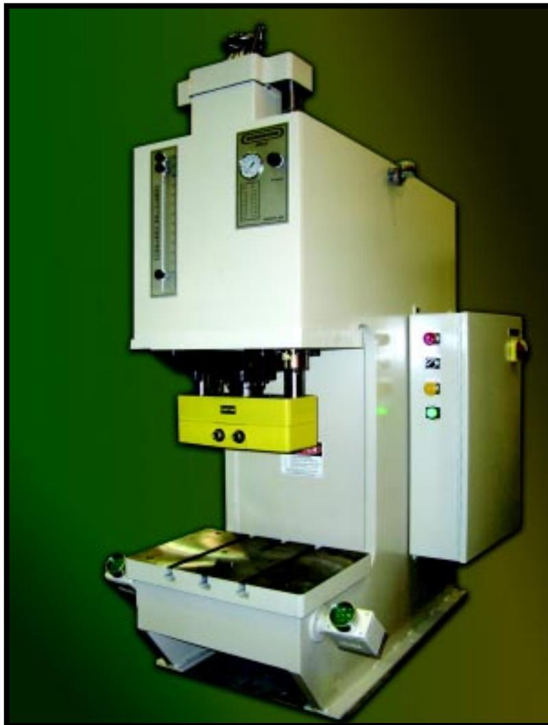
Pressure easily adjustable on up-front control panel.
