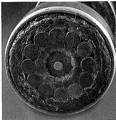
Left: Fragment of the 1863 Persian Gulf cable manufactured by Henleys Telegraph Works Co. Ltd. "Two servings of hemp" were added for strength, according to a Globe article at the time.
