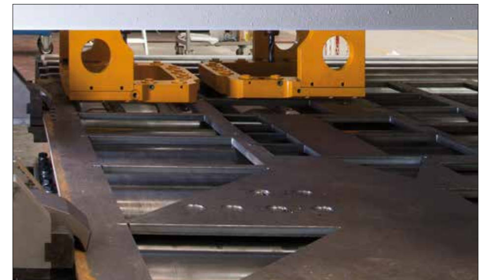
Lateral material clamps and dual spindle configuration
