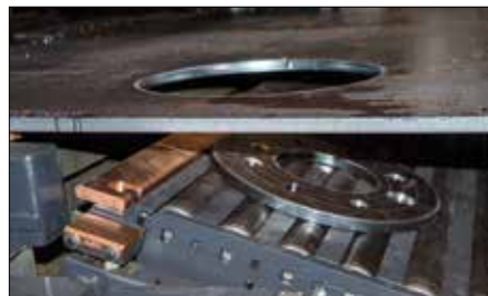
Trap door for part unloading
