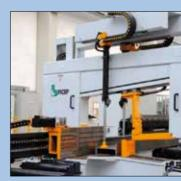
Automatic unloading device with magnet
